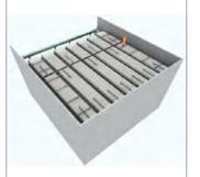
**7.** The outer line of Quad-Lock ICF panels are extended above the level of the poured concrete floor and braced.
