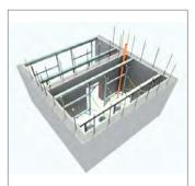
**2.** Support system is setup at right angles to the direction of the Quad-Deck flooring panels.
