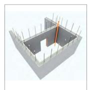
1. Walls are prepared and checked to be level and cleared of any debris. Steel work is left projecting up to 1m.
