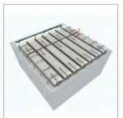
**6.** Steel meshing is placed on top of the bent steel and tied with wire to securely fix in position.
