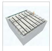
**5.** Steel bars are bent 90° over the Quad-Deck panels and lengths laid on mounts between each board.
