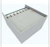
**8.** The concrete is poured over the panels to a thickness of between 38 - 150mm and finished as required.
